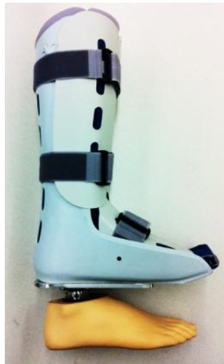
Fig. 2: Pneumatic walking brace with prosthetic foot mounted below.
