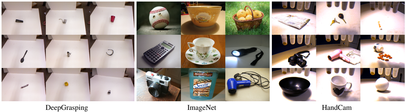
Fig. 2: We use three datasets to evaluate our system: Deep Grasping, ImageNet, and HandCam. Because of bias towards power, pinch, and three jaw chuck in Deep Grasping, we chose to create a dataset from ImageNet that more uniformly represents all five grasps. We then created the HandCam dataset from images captured by our hand camera to test the validity of our system.
