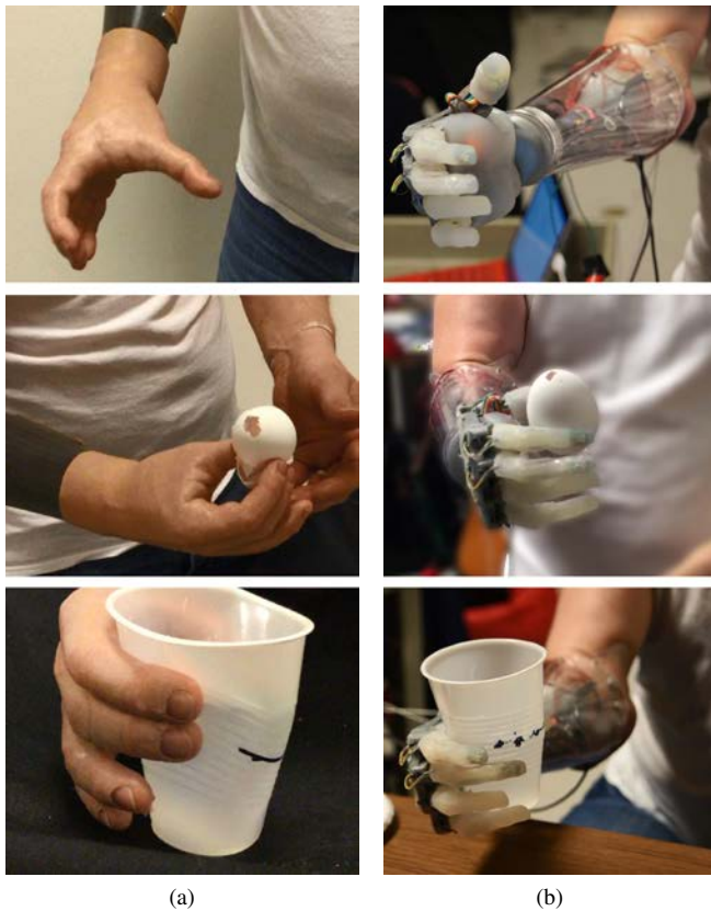
Fig. 4. Experiments with (a) the subject’s original myoelectric prosthesis showing him crushing the egg and cup. However, when using the new hand as shown in (b), he successfully grasps the egg without cracking it and grips the cup with minimal water displacement.
